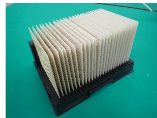
Figure 4. Assembled PCBs Stored in a PCB Holder
