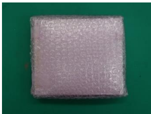
Figure 5. Assembled PCB that is Wrapped with Antistatic Bubble Wrap
